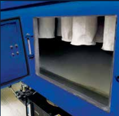
Larger baghouse access doors
